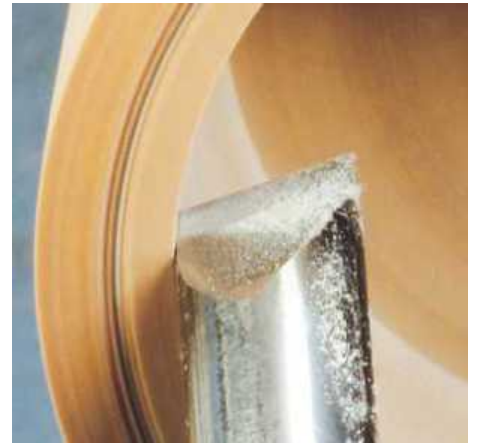
STEP 15. The round skew is so good at making light shearing cuts to achieve a good finish. The side of the tool will just remove tiny amounts of shavings and will leave the surface needing little sanding
